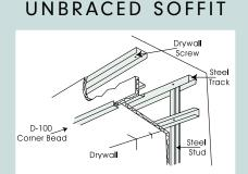
Note: For typical applications maximum width and or height should not exceed 24".
