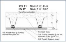
**NOTES ON ACOUSTICAL PERFORMANCE**: Acoustic tests are based on **ASTM E90 (STC)** and **ASTM E492 (IIC)**. Sound loss and sound transmission are measured by a series of instruments from which the ratings are calculated for design.
